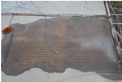
Figure 6: Surface heating trial with copper wire from Heymsfield et al. (2012) study.
