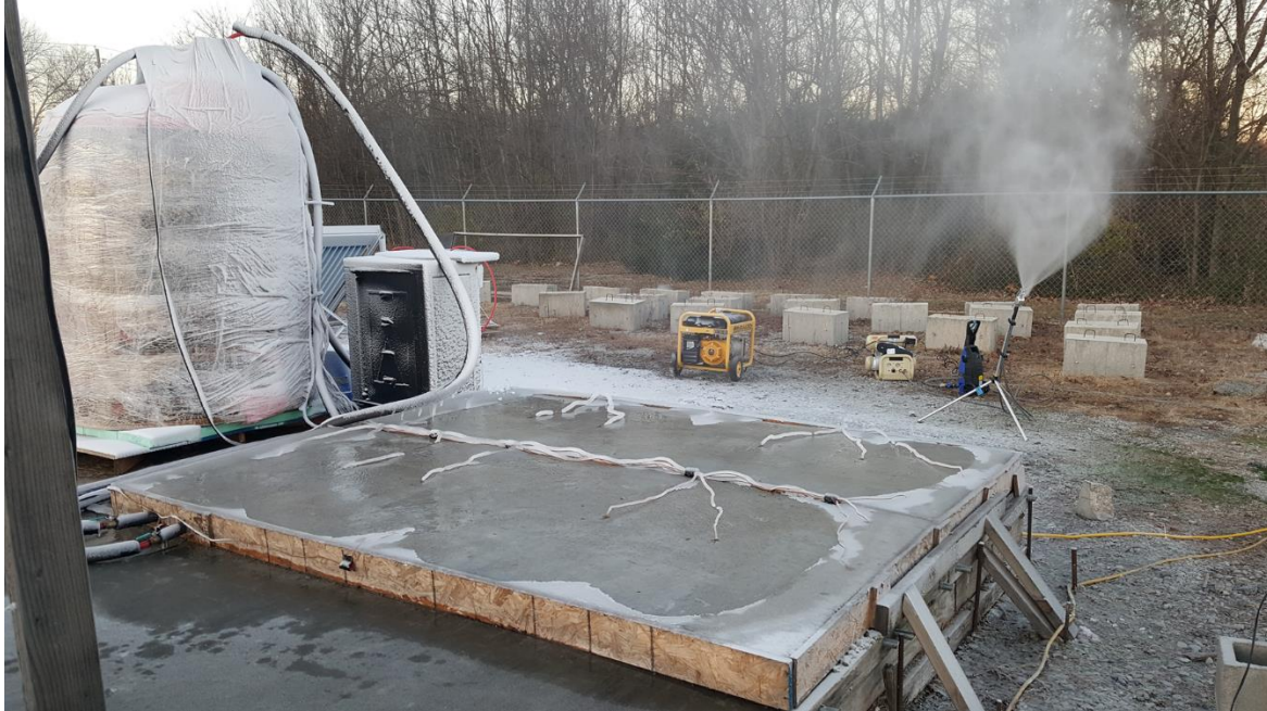
Figure 111: Snowmaking machine positioning for anti-icing tests.
