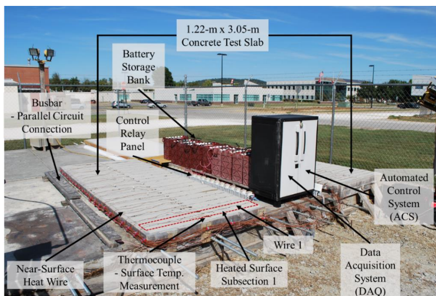
Figure 31: Large-scale test site configuration.
