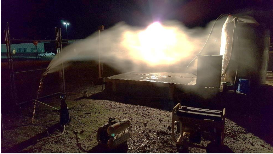
Figure 42: Manmade snow with a snowmaking machine.
